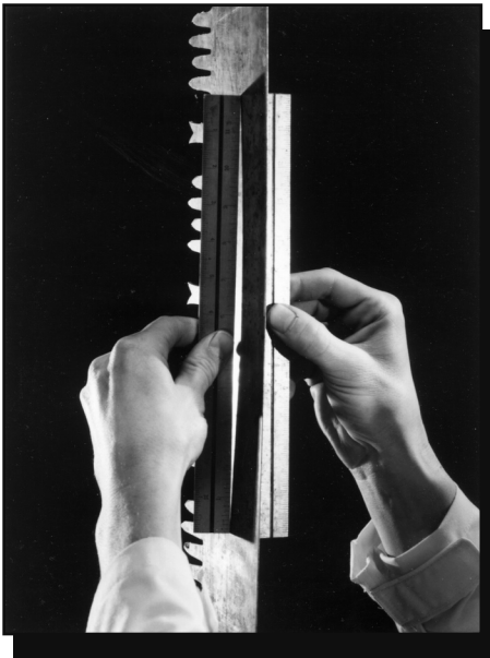
Figure 18—Locating kinks with two straightedges.
