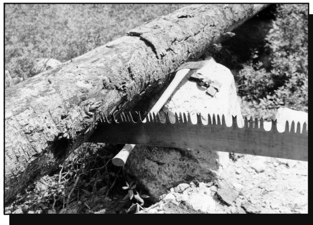
Figure 50—An ax planted in the lower part of the log can work as an underbuck.
