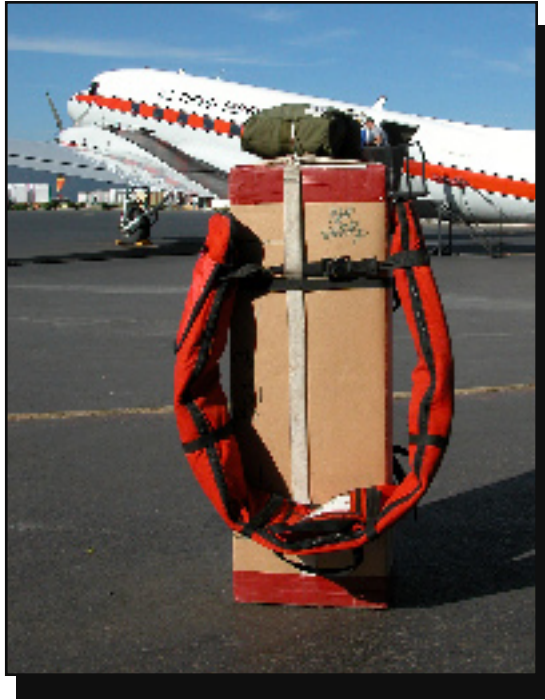
Figure 29—A crosscut saw rigged for a parachute drop.
