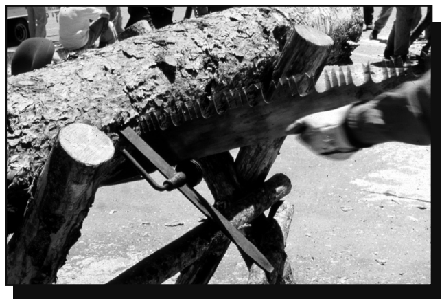
Figure 42—This vintage mechanical underbuck helps hold the saw up so it can cut from beneath the log. This is one design of many that were available.
