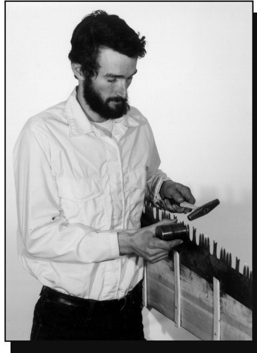
Figure 26—Warren Miller setting cutter teeth.
