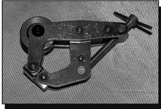
Figure 43—The MTDC underbuck features a 2-inch clamp with a shielded steel pulley. It attaches to an ax handle.
